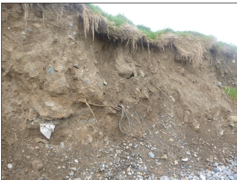
Photo 3-21 SP10 - C&D Material 'made ground' in cliff face
