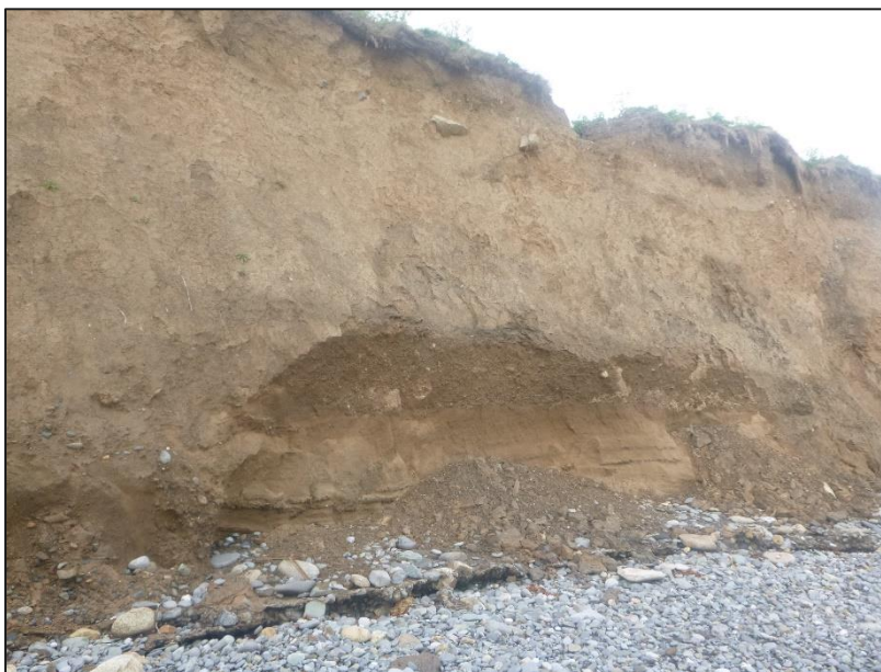
Photo 3-15 SP7 - Section of cliff face failure in sand and gravel material with slumping
